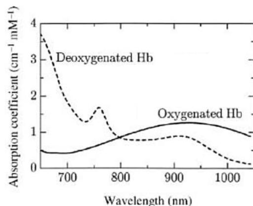
Fig. 1. Absorption spectrum of oxygenated and deoxygenated hemoglobin (Hb) [1]
