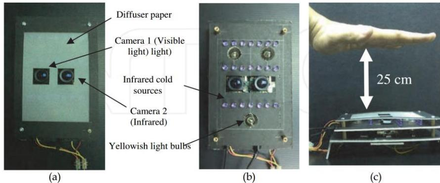
Fig. 6. (a) Image acquisition device (covered). (b) Image acquisition device (uncovered). (c) Acquiring the hand images.
