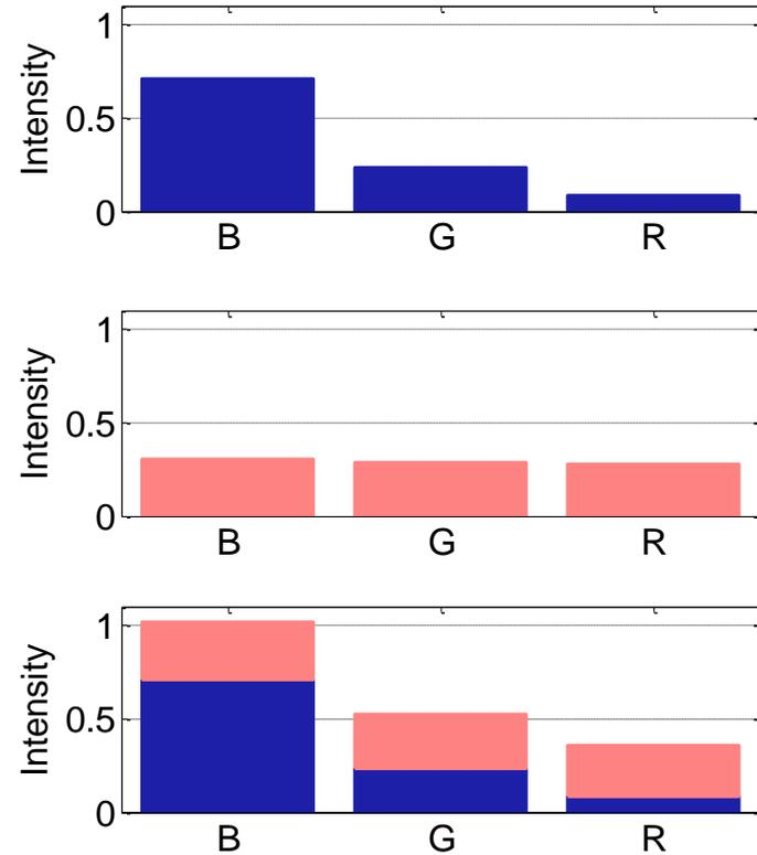
Illumination intensities determine feature information distribution in color channels. Feature of each modality can be pronounced in its own color channel.
