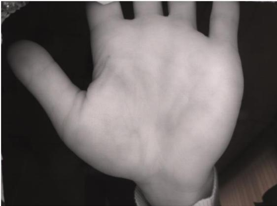
Palm vein images, obtained using 850 nm band-pass filter
