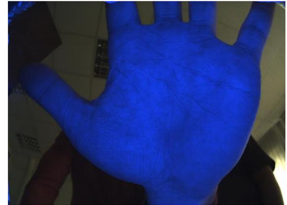
Palm ridge images, obtained using near-infrared light band-stop filter
