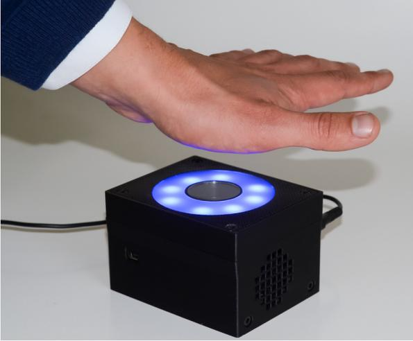
Figure 2. Picture of the developed FPGA-based palm biometric system prototype
