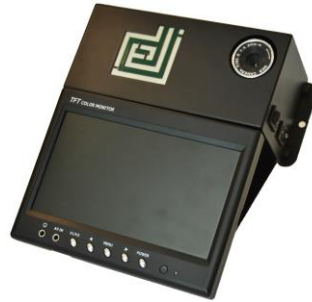
Fig.8: Developed face recognition system
